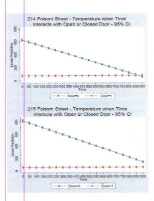
Very similar results that reveal temperatures reduce over time in the rooms with open doors, but the initial temperatures were high enough that the fire event was not survivable. The rooms with the doors closed remain survivable throughout the fire event.<sup>1</sup>
