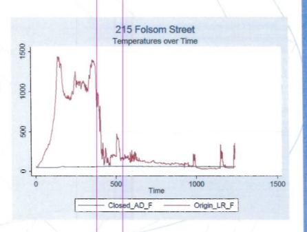
seconds (time) are from the closed door bedroom and the last 917 seconds (time) from the living room. In test 2 (215 Folsom Street) the first 1,241 seconds (time) are from the closed door bedroom and the last 1,241 seconds (time) from the living room.
